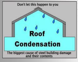
**Vapor Control** - We offer a range of vapor retarder facings applied and ready for installation. Facings with a maximum permeance rating of 0.1 perm are recommended for optimum moisture condensation control. Detailed performance and physical property data concerning available facings is available from facing manufacturer.
