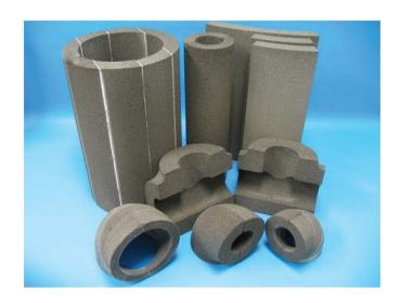
Pipe, fittings, curved segments, precision machined tank heads and basic block insulations are supplied for a wide variety of above and underground applications. Cellular Glass insulation sections are fabricated with reactive gypsum or bituminous adhesive.
