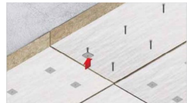
Install lock washers
